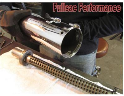
**Step 5** - Debur the saw cut and drill holes.
