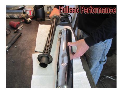
**Step 6** - Test fit the core by aligning the inlet cut away with the muffler indentation. The new core should fit tight but still slide in by hand. If not, additional filing at the saw cut edge may be required to open the saw cut end. Do not hammer the core in!
