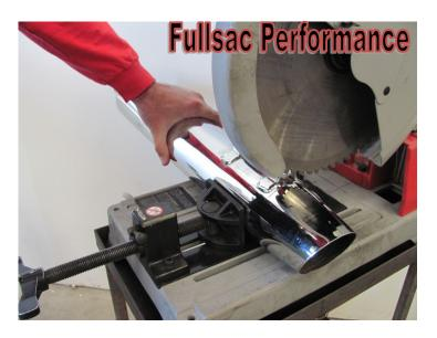
**Step 1-** Using a chop saw, band saw, or sawzall, cut the exit end off the muffler as close to the weld as possible. Don't worry if your saw cut is not perfectly straight. The end cap will cover it. It is important to remove all of the tapered section. You need a clean 4" opening to insert the new core.
