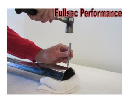
**Step 3** - Center punch as close as possible to the center of your felt pen mark. Don't worry if you're off a little. Misalignment can be corrected during drilling
