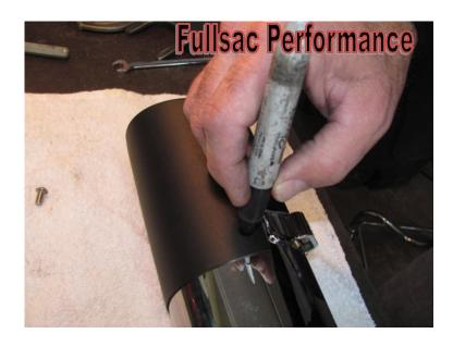
**Step 2** – Remove all packing material from your muffler. Slide your new end cap over the end of your muffler. Push it all the way on as far as possible. Rotate it left and right and center it up. Using a sharpie felt pen, mark the three holes.
